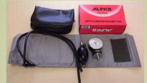
Manometer: 0—300mm Hg, with zero stop pin
